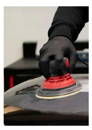
The Mil P600/800 grits are created to opacify the supports during the painting and shading phase of the transparent varnish; the Mil P1200 grain, on the other hand, was created to remove serious defects such as scratches, orange peel and acid defects from all external painted supports.
